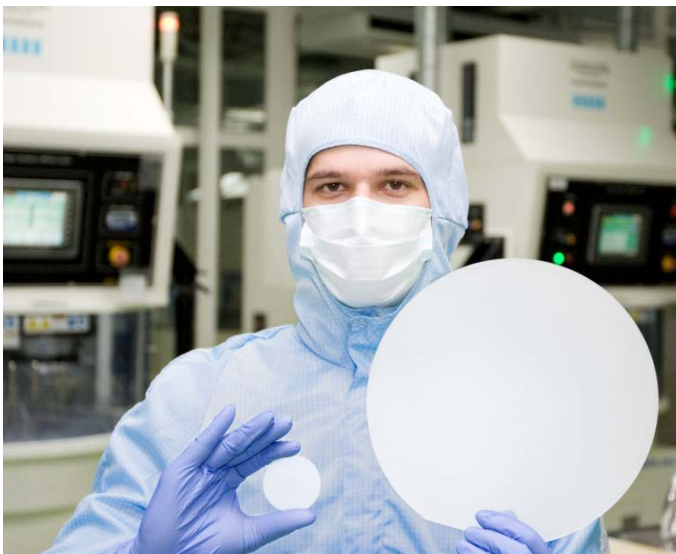
Monocrystal's 10-inch sapphire substrate vs 2-inch sapphire substrate
